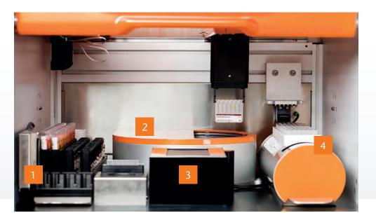
Sample and reagents area with 32 positions for sample tubes and 20 positions for reagents
