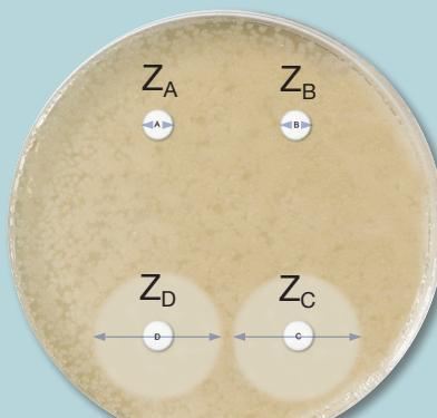
$Z_D - Z_B$  and  $Z_C - Z_A \geq 5\text{mm}$
